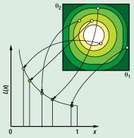
1: A schematic of the nested sampling algorithm. The 2-D parameter space is shown at the top right. The points within it are considered to represent contours of constant likelihood, which sit within each other like layers of an onion (there is, however, no need for them to be simply connected). The volume corresponding to each thin shell of likelihood is computed by the algorithm, allowing the integral for the evidence to be accumulated as shown in the graph.
