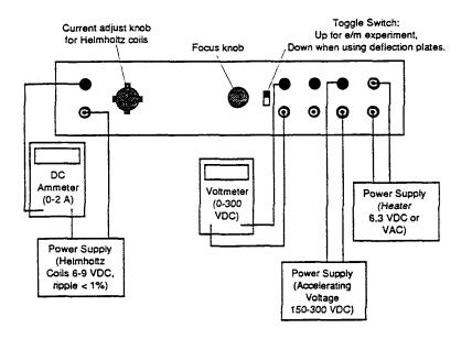
Figure 3. Connections for e/m Experiment
