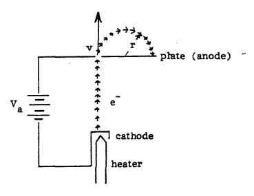
Figure 1. Electron trajectory in the e/m apparatus.
