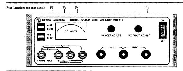
The PASCO scientific Model SF-9585 High Voltage Power Supply provides regulated DC power up to 50 mA in two voltage ranges: 0 to 50 and 0 to 500 volts. The output for the two ranges are independently adjustable, though a single terminal is used as the positive terminal for the 50 volt output and as the negative terminal for the 500 volt output. The meter may be switched to read current or voltage in either range.
