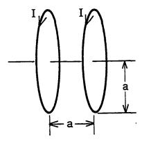
Figure 4. Helmholtz coil arrangement.
