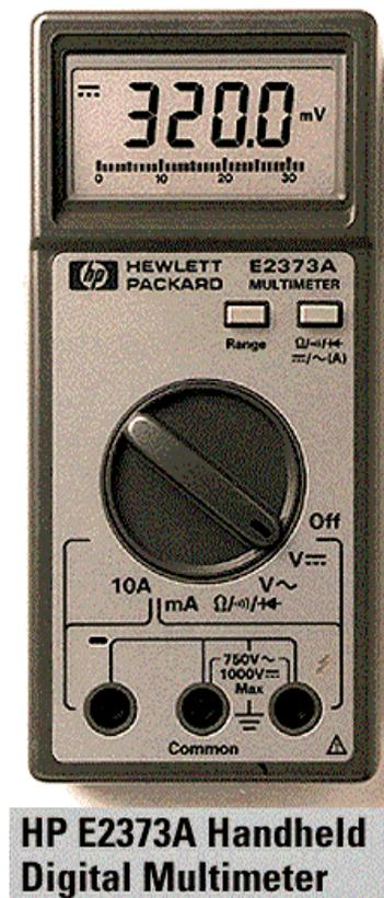
**HP E2373A Handheld Digital Multimeter**
