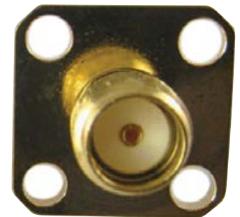
1. The SMA connector is one of the most common connector types used for RF/microwave applications.
