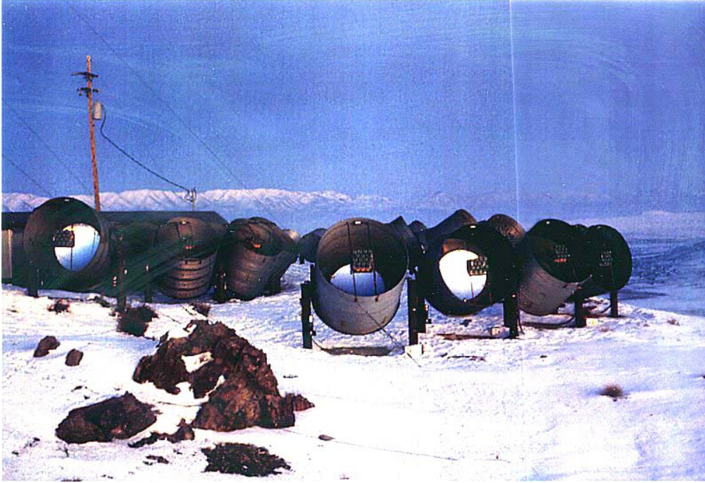
Figure 3: The Fly’s Eye array operated out of Dugway Proving Ground, a military base in the desert of western Utah, from 1981 to 1993; it pioneered the “air fluorescence technique” for determining the energies and directions of ultrahigh-energy cosmic rays based on faint light emitted by nitrogen air molecules as the cosmic-ray air shower traverses the atmosphere. In 1991, the Fly’s Eye detected a cosmic ray that still holds the world record for highest-energy particle (from https://www.quantamagazine.org/the-particle-that-broke-a-cosmic-speed-limit-20150514 ).
