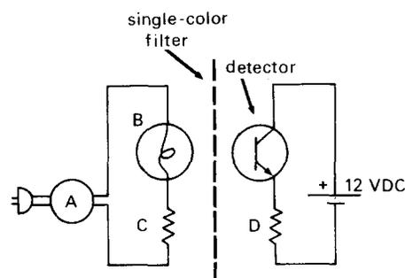
Fig. 1. Planck's constant experiment. Variac ( $A$ ) delivers two different powers to filament ( $B$ ). These powers and their corresponding two photocurrents through the detector<sup>5</sup> are determined with a roving ac/dc voltmeter, applied across  $B, C$ , and  $D$ .
