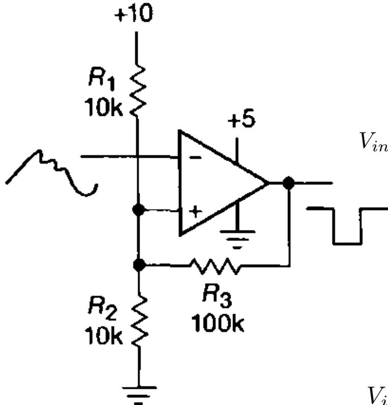
$$\text{SE } V_{\text{O}} = 5V \quad \frac{V_{\text{in}} - 10V}{R_1} + \frac{V_{\text{in}} - 5V}{R_3} + \frac{V_{\text{in}}}{R_2} = 0$$
