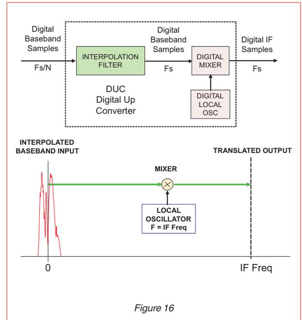
Figure 16 is a frequency domain view of the digital upconversion process.
