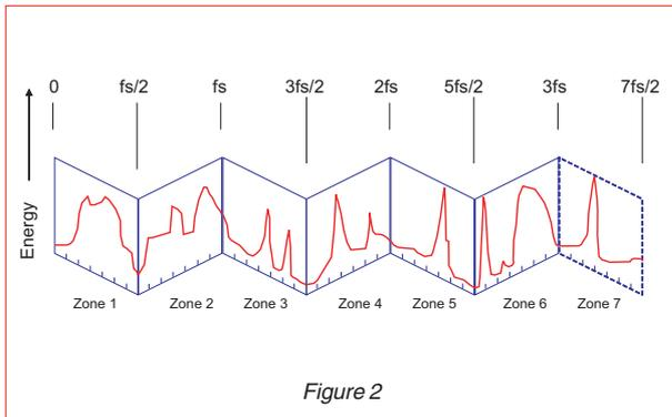
Use the vertical axis of the fan-fold paper for signal energy and plot the frequency spectrum of the signal to be sampled, as shown in Figure 2. To see the effects of sampling, collapse the transparent fan-fold paper into a stack.
