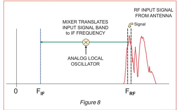
The mixer performs an analog multiplication of the two inputs and generates a difference frequency signal.
