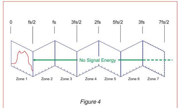
A baseband signal has frequency components that start at  $f = 0$  and extend up to some maximum frequency.
