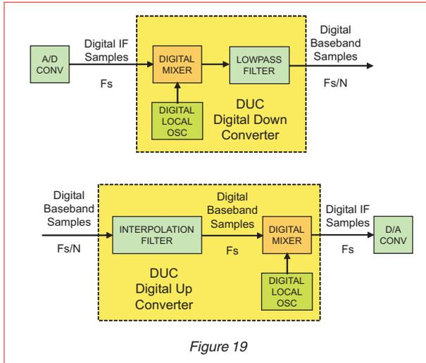
Think of the DDC as a hardware preprocessor for programmable DSP or GPP processor. It preselects only the signals you are interested in and removes all others. This provides an optimum bandwidth and minimum sampling rate into the processor.
