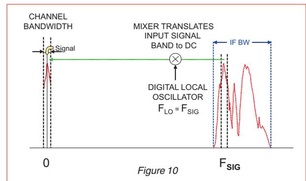
At the output of the mixer, the high frequency wideband signals from the A/D input (shown in Figure 10 above) have been translated down to DC as complex I and Q components with a frequency shift equal to the local oscillator frequency.
