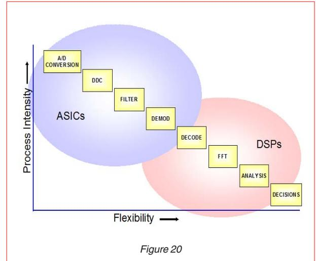
Here we've ranked some of the popular signal processing tasks associated with SDR systems on a two axis graph, with computational Processing Intensity on the vertical axis and Flexibility on the horizontal axis.
