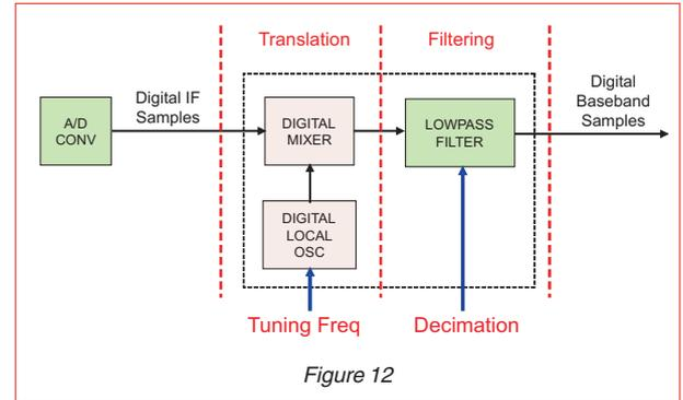
This process is called *decimation* and it means keeping one out of every N signal samples. If the decimated output sample rate is kept higher than twice the output bandwidth, no information is lost.
