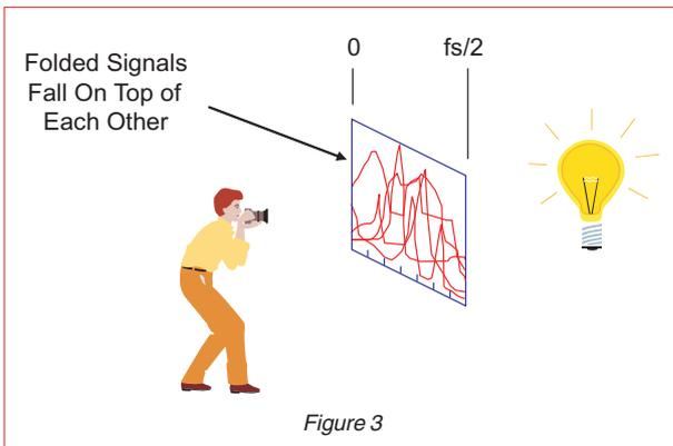
The resulting spectrum can be seen by holding the transparent stack up to a light and looking through it. You can see that signals on all of the sheets or zones are “folded” or “aliased” on top of each other — and they can no longer be separated.
