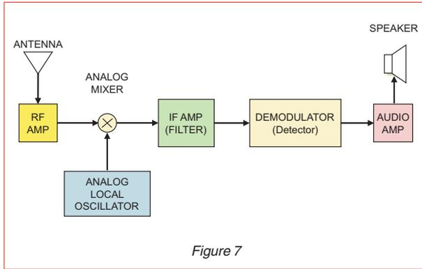
The conventional heterodyne radio receiver shown in Figure 7, has been in use for nearly a century. Let's review the structure of the analog receiver so comparison to a digital receiver becomes apparent.
