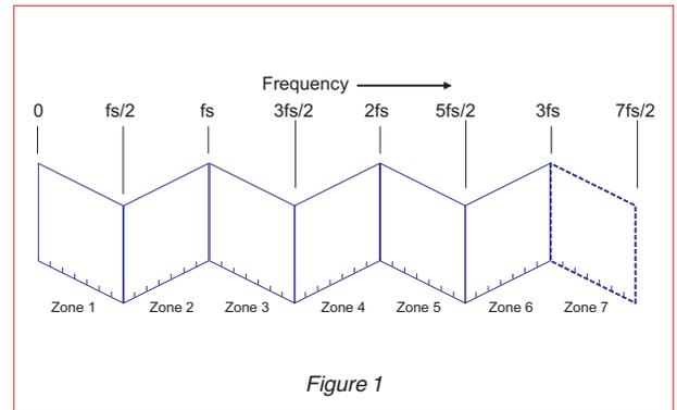
To visualize what happens in sampling, imagine that you are using transparent "fan-fold" computer paper. Use the horizontal edge of the paper as the frequency axis and scale it so that the paper folds line up with integer multiples of one-half of the sampling frequency  $f_s$ . Each sheet of paper now represent what we will call a "Nyquist Zone", as shown in Figure 1.
