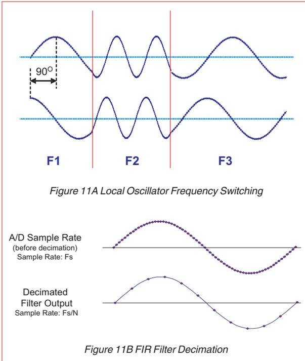
Because the local oscillator uses a digital phase accumulator, it has some very nice features. It switches between frequencies with phase continuity, so you can generate FSK signals or sweeps very precisely with no transients as shown in Figure 11A.
