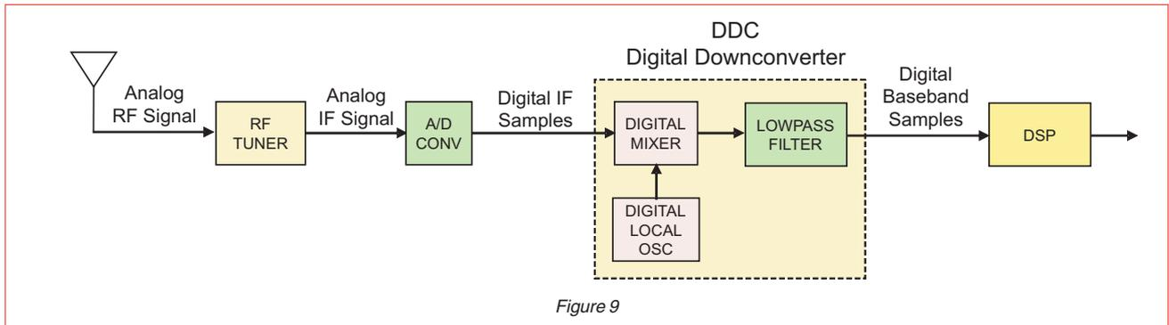
Figure 9 shows a block diagram of a software defined radio receiver. The RF tuner converts analog RF signals to analog IF frequencies, the same as the first three stages of the analog receiver.
