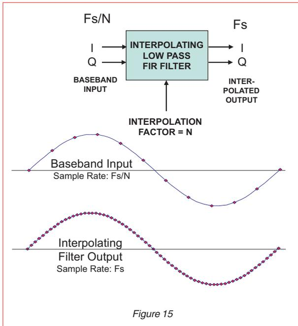
The interpolation filter must boost the baseband input sample frequency of  $f_s / N$  up to the required mixer input and D/A output sample frequency of  $f_s$ .
