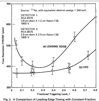
Timing for a Narrow Pulse-Height Range. The source was <sup>22</sup>Na, with the selected equivalent electron energy in the scintillator = 340 keV. The time resolution (FWHM) is Δt.
