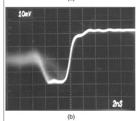
Fig. 12. Monitor Signals when Triggered by the Constant-Fraction Discriminator Output Signal for (a) Passive Pulse Shaping and (b) for Active Pulse Shaping.
