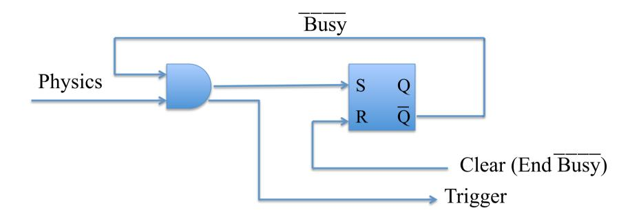
The arrival of a "Physics" event will generate a "Trigger" signal which is sent to the computer. At the same time the Trigger will inhibit the coincidence to future events by setting the "Busy-bar" signal (which will go to "zero"). The coincidence will remain inhibited until a Clear signal is sent by the computer which will end the Busy-bar signal and open the coincidence to future Physics events.
