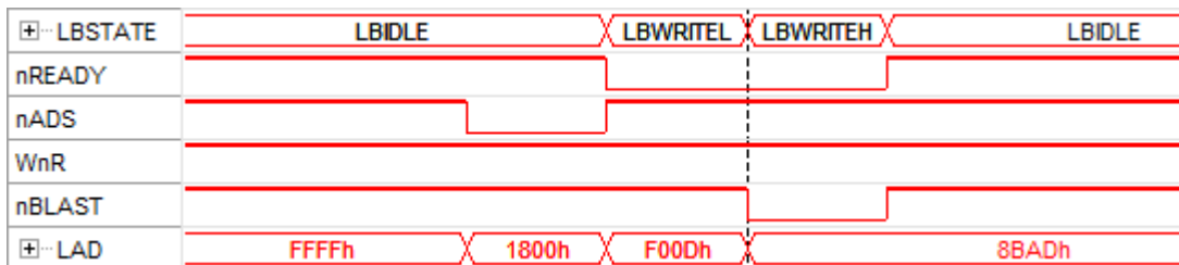
Fig. 13.3: Local bus signals at a write access (x8BADF00D is written on register x1800)
