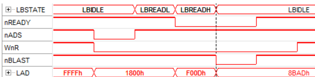
Fig. 13.4: Local bus signal at a read access (x8BADF00D is read from register x1800)
