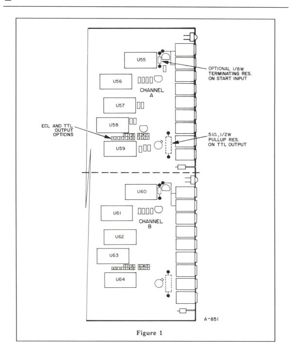
Should the user wish to terminate the START input with a resistor to ground (typically 50  $\Omega$ ), space is available at the frontpanel side of U55 (U60), the AM865's, for an 1/8 W resistor.
